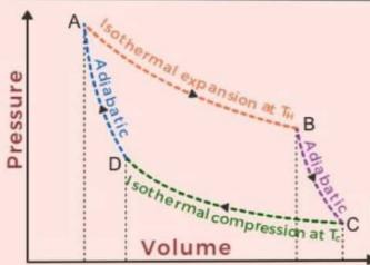
A Carnot heat engine is an engine that operates on the reversible Carnot cycle. The basic model for this engine was developed by Nicolas Léonard Sadi Carnot in 1824.
